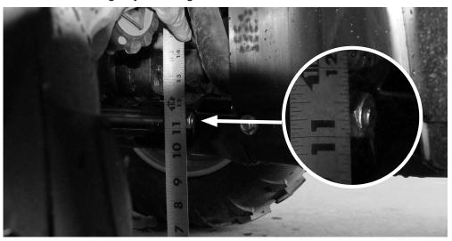
**Front Suspension:** Measure the height from the floor to the center of the front lower rear a-arm mount. The standard height is **11.250 - 11.500 inches**. Ensure this is equal from side to side on the vehicle. Adjust spring preload to obtain these measurements.
