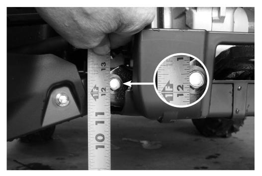
**Rear Suspension:** Measure the height from the floor to the center of the rear lower a-arm mount. The standard height is **12.250 - 12.500 inches**. Ensure this is equal from side to side on the vehicle. Adjust spring preload to obtain these measurements.
