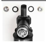
O-rings and reducers are pre-installed in the upper mounting positions. Bushings and sleeves are pre-installed in the lower mounting positions. When mounting all shock absorbers, position the rebound adjusters to face the ATV's wheels.
