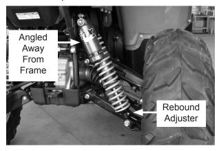
**Rear shocks:** The Yamaha Grizzly rear shocks are left and right specific. When mounted correctly, the piggyback reservoir end of the shock will be connected to the frame with the reservoir facing the rear of the vehicle and angled away from the frame. The lower shock eyelet will be connected to the a-arm with the adjuster facing the wheel, as shown above. Torque all mounting hardware to the vehicle manufacturers specifications.
